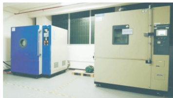
Low pressure test box (left) Constant temperature and humidity test box (right)
