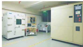
Natural convection test box (left) Cold and hot shock test box (right)
